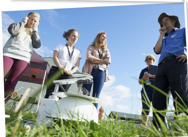
Professor Louis Schipper (University of Waikato) describes automatic chambers in the foreground that measure carbon dioxide coming out of the soil.
