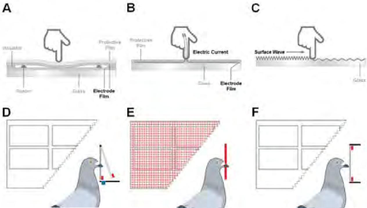
**Figure 6.** Resistive (A), capacitive (B), and acoustic wave touch screens (C). Flappy key (D), infra-red (E) and pressure sensitive (F) key setups.
