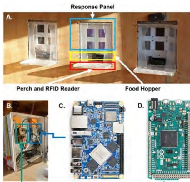
**Figure 3.** The response panels that face into the pigeon loft (A), behind the response panels is an LCD screen used to display stimuli (B), a NanoPC-T4 used to control the stimulus display (C) and an Arduino Due microcontroller that controls the administration of food (D).
