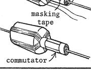
Make 2 BRUSHES as shown. Attach these to the base board so they just touch the commutator wires.
