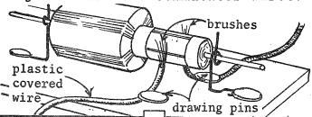
Wind about 20 - 2 turns of copper wire around the cork.
